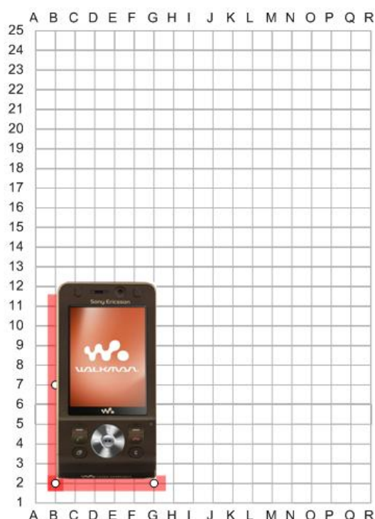
Rohde & Schwarz Coupler with a Grid Positioning plate Reference point B2
